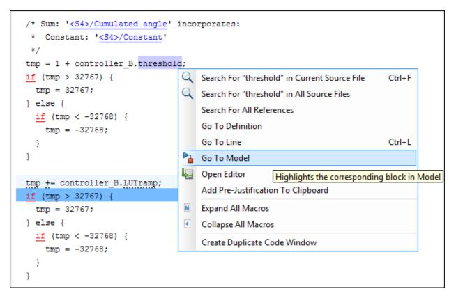
The model shows the corresponding block highlighted in blue. If the block is in a subsystem, both the subsystem and the block are highlighted in blue.
