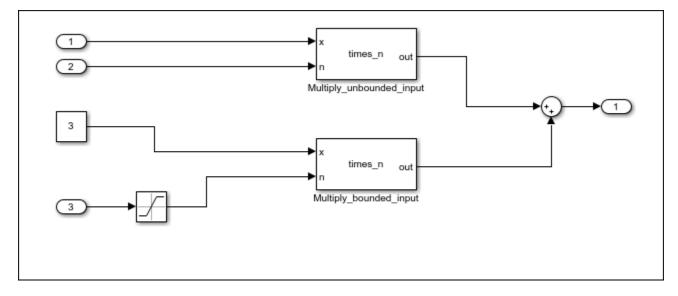
When you analyze custom code, in this case the function times\_n, the analysis shows that an operation in the custom code can overflow. From the analysis results, you can determine that the
